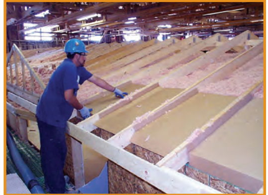
Building in a climate controlled environment reduces costs by protecting materials from the elements
